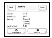
The **status** screen provides several items of information about the current operation status of the CP-500, as well as access to information on the software used in and the internal sensors of the CP-500.
